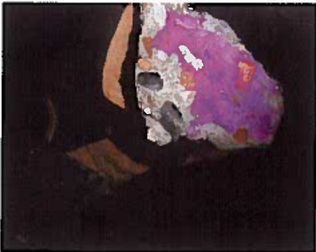
Figure 2: Pink concrete is toward the center of the member and not contaminated by carbonation.
